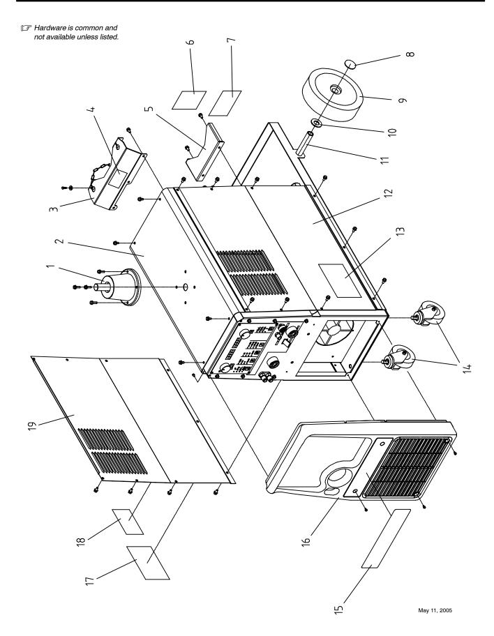
Figure 7-1. Unit Outer Assembly
